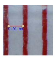
2) Multi-line: click, left-click mouse to choose a start point and drag to an end point. Notice that the measurements are displayed as you go along. Release mouse when done. You can continue measuring from the previous end point to a next point and so on.
